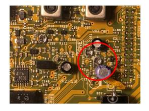
Press the PTT and carefully adjust the deviation control pre-set to the desired value.
