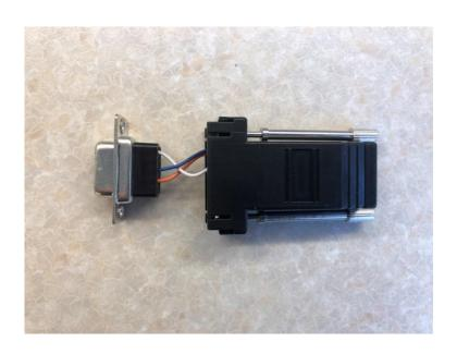
Carefully snap the socket into the housing, the adaptor should now look like this.
