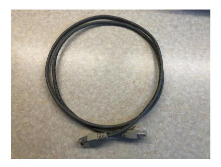
Note 4\_ KM3000 4000 RJ45 type programming conector
