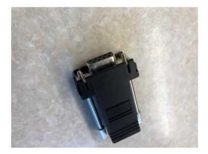
Plug a standard CAT5 RJ45 patch lead (not a cross-over) into the oposite end of the adaptor and the other end into the radio socket. Plug the adaptor into the PC serial port or USB to serial adaptor. The radio can now be programmed. If the radio (some KM4000's) has a male RJ45 plug fitted the plug can be used straight into the adaptor without the patch lead.
