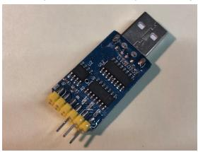
3. Then cut the remaining three pins short leaving about 3mm exposed.
