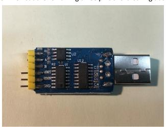
5. There are three small switches on the PCB selecting the RS232 setting. The top switch needs to be in position 2, the bottom switch to the ON position, and the single vertical switch which is to the left of where DTR is printed on the PCB to the UP position towards the edge of the board.
