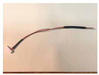
7. Strip and tin the ends ready to solder the wires to the module.
