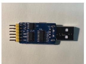
2. Carefully remove the unused pins to leave just the three RS232 pins (232T, 232R and GND).
